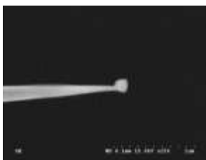
Figures: Left: SEM image of a fluorescent-SThM tip; Right: topography and thermal images measured on a nanostructured microwire, hot spots are visible at every constriction.
